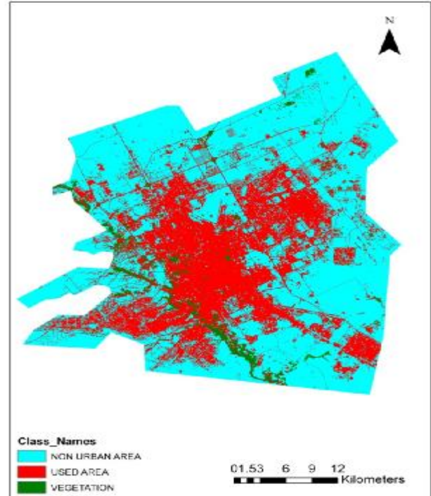
Fig.9. Classified image of 1994 with scale parameter of 10, shape factor of 0.3 and compactness of 0.5 (level 1). The classification method was achieved by nearestneighbour classification method.
