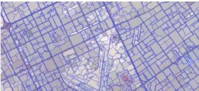
Fig.5. Example of segmentation view with scale parameter of 35, shape factor of 0.5 and compactness of 0.5 (level 2).
